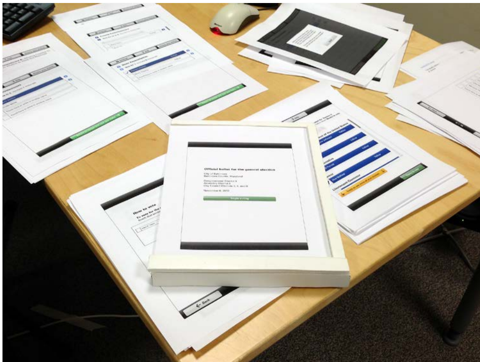
The “tablet computer” to be used by the participant in paper prototype testing, with the first screen of the ballot showing.
